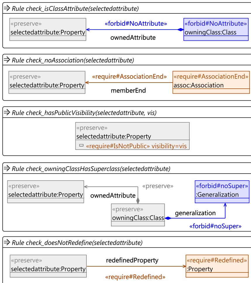
Figure F.35: Initial Check Implementation of UML class model refactoring Pull Up Property
