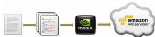
Figure 1. GPU-based Cloud computing for structural analysis of protein binding sites: sequential C++ program, parallel OpenCL program, single GPU execution, multi GPU-based Amazon Cloud execution.
