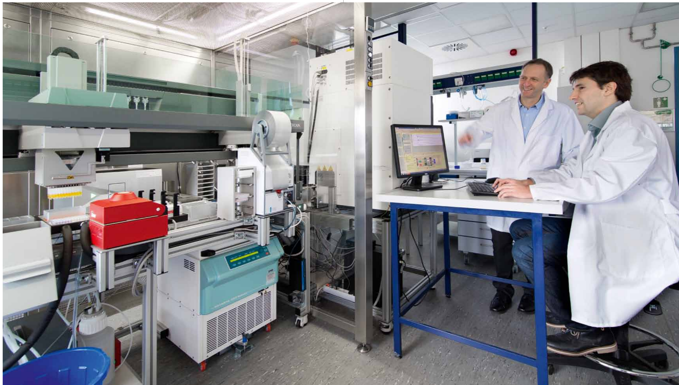
The Tecan Freedom Evo automation platform with its numerous integrated laboratory devices, such as PCR machine, multimode reader, sealer and centrifuge.
