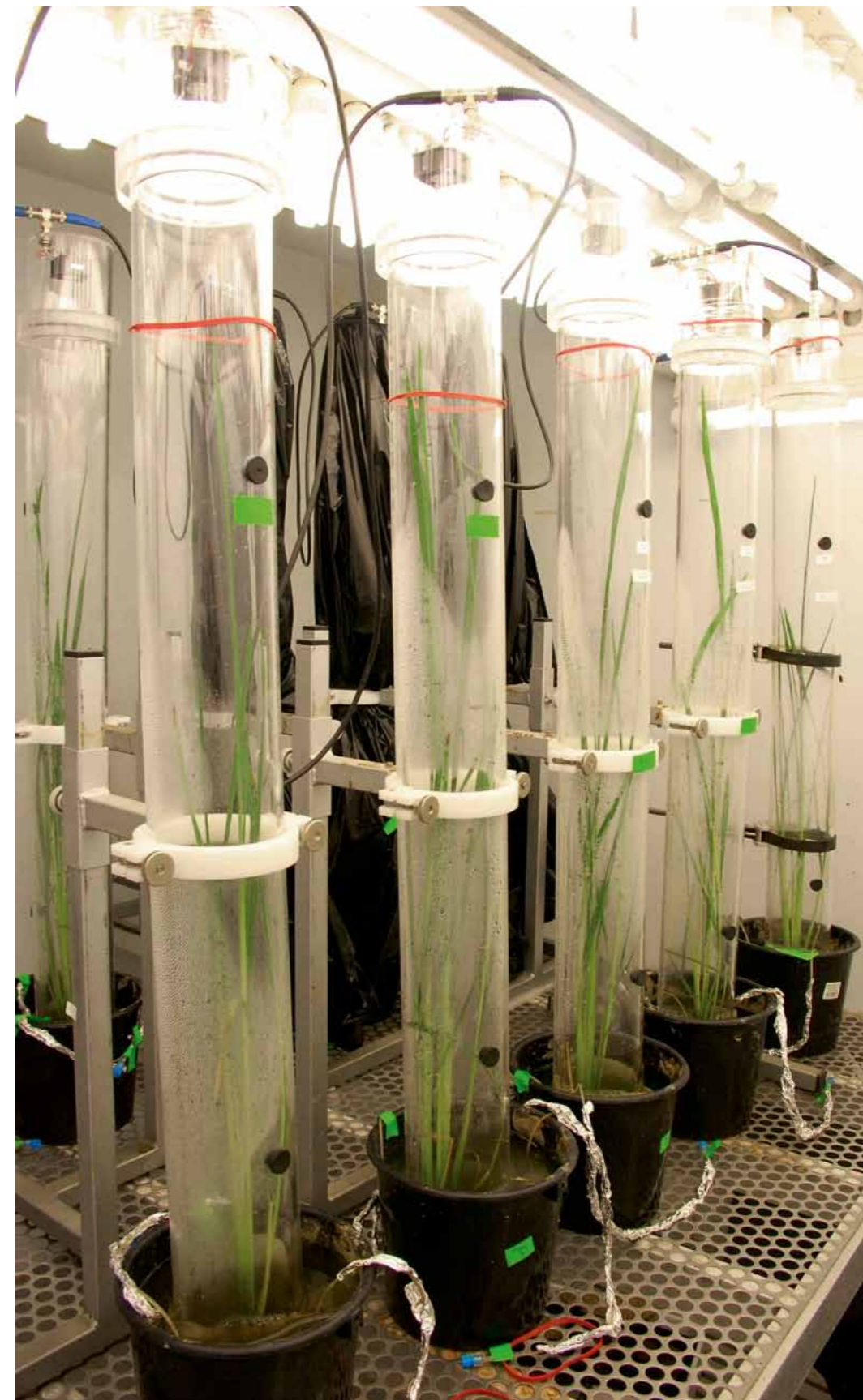
Figure 2. Device for pulse-labeling of rice microcosms with ^{13}\text{CO}_2 and measuring the flux of \text{CO}_2 and \text{CH}_4 between the microcosms and the atmosphere. (Photo: Judith Pump)
