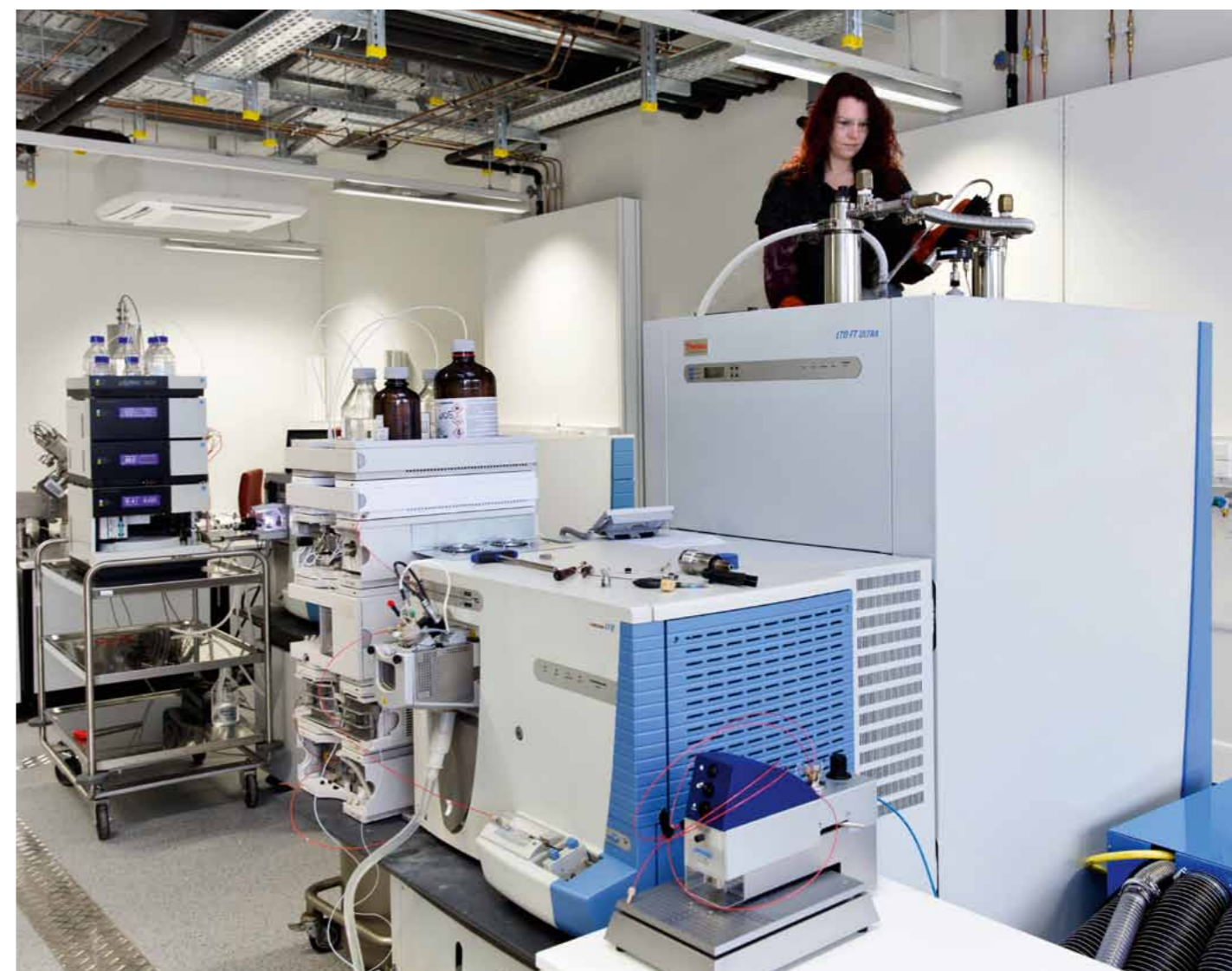
Filling liquid nitrogen into the supra-conducting magnet of the LQ-FT Ultra mass spectrometer. The nano-RSLC seen in the back is coupled to an Orbitrap Velos Pro mass spectrometer.
