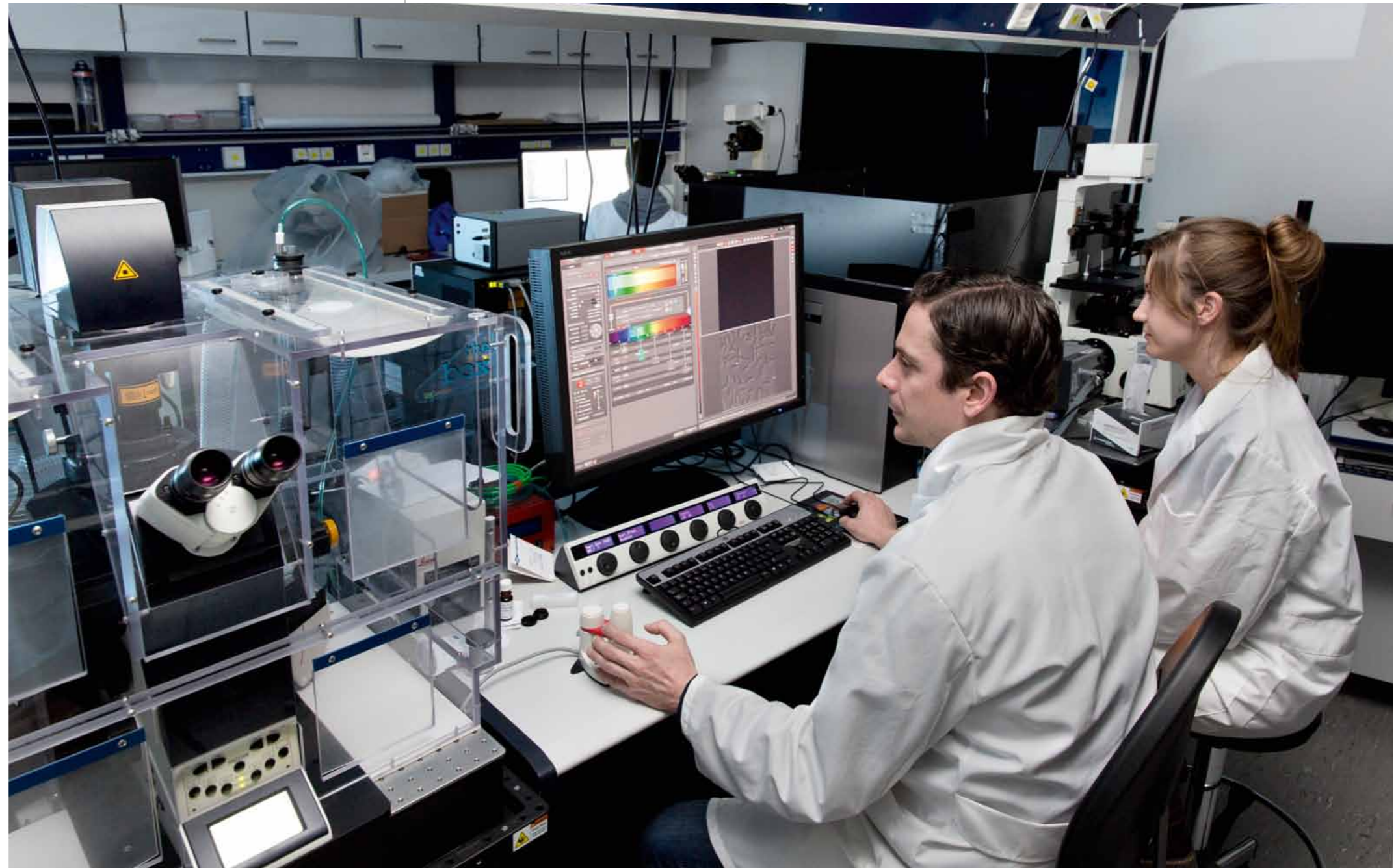
The stimulated emission depletion super resolution scanning confocal microscope (Leica, TCS SP8 STED).
