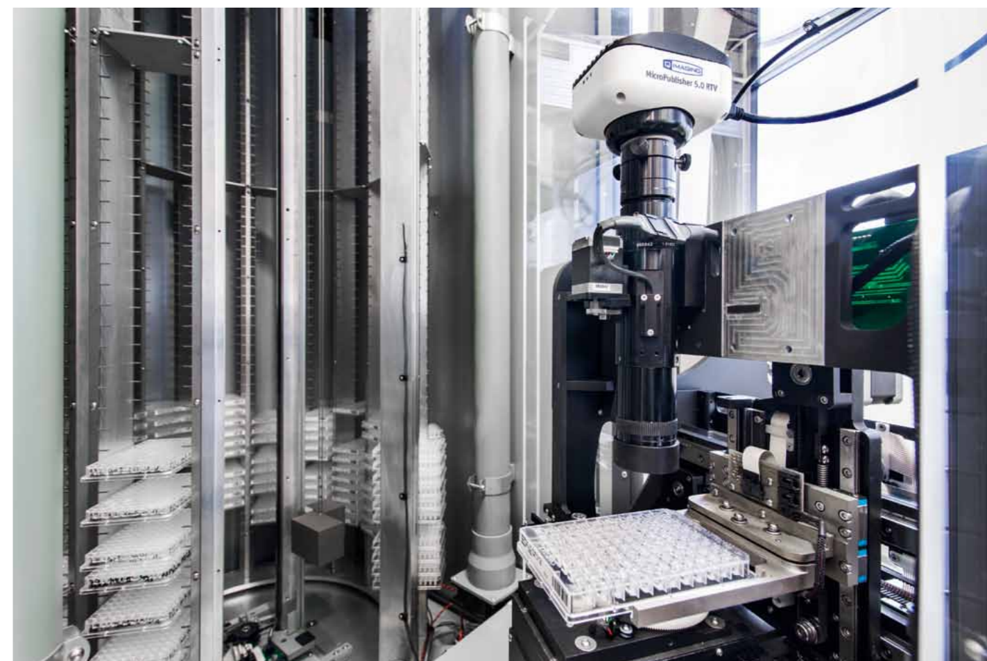
One of the Formulatrix Rock Imagers™ with incubator (left) and imaging unit (right).
