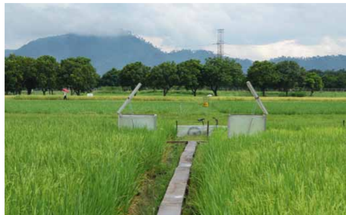
Figure 1. Rice field in the Philippines with flux chambers for measuring \text{CH}_4 emission. (Photo: Ralf Conrad)
