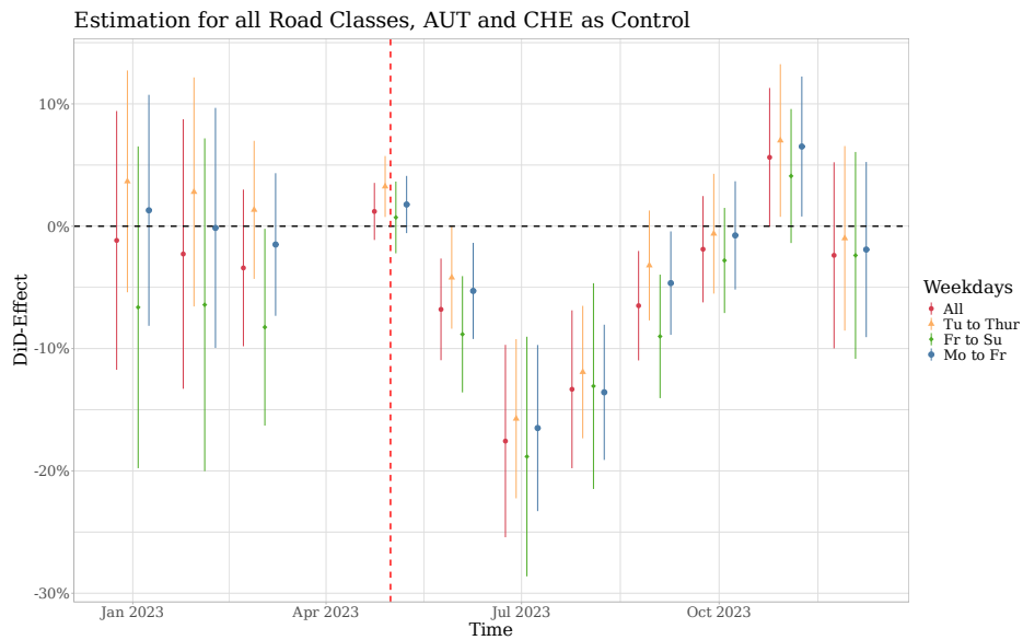
Figure B.3: Event Study results based on Equation (2). The dependent variable is the logged car traffic on freeways and highways (using 95% confidence intervals). The vertical red line marks the introduction of the Deutschlandticket . April 2023 serves as the reference period.
